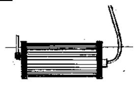
filter is completely down in the solution and filled with solution let it swim. Connect the other end of the suction tube at the pump suction side.
