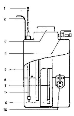
The dissolving water coming from any pressure system > 0,5 bar (from filter or drinking water supply tubing) is conveyed to the bottom of the Turbo-Dissolver to a
